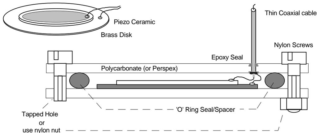
**Note** - for new ceramic disks - When soldering connecting wires to the silvered ceramic surface clean the joint surface very carefully (scrape lightly with a scalpel). Use a
